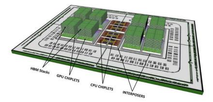
Figure 11.9: AMD's chiplet-based architecture.
