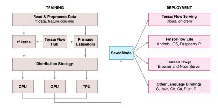
Figure 7.16: Architecture overview of TensorFlow 2.0. Source: Tensorflow.
