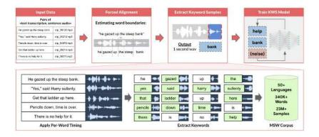
Figure 6.15: MSWC's automated data labeling pipeline.
