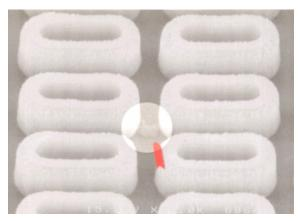
Figure 18.12: Residue induced intermittent fault in a DRAM chip. Source: Hynix Semiconductor
