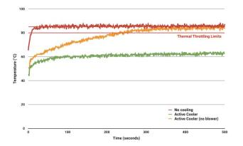
To prevent overheating, all Raspberry Pi boards begin to throttle the processor when the temperature reaches 80°Cand throttle even further when it reaches the maximum temperature of 85°C (more detail here).
