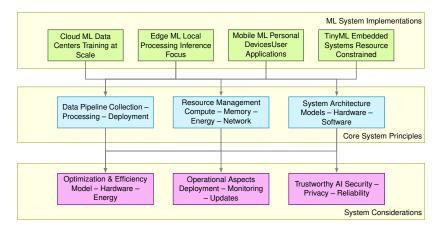
Figure 2.11: Core principles converge across different ML system implementations, from cloud to tiny deployments, sharing common foundations in data pipelines, resource management, and system architecture.
