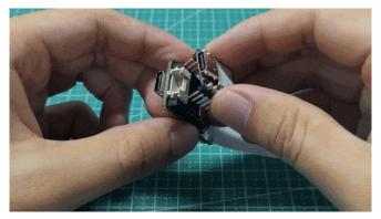
**CAUTION**: Please note the direction of the connection, Grove Vision AI's Type-C connector should be in the same direction as XIAO's Type-C connector.
