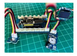
The Grove Light Sensor would be connected to one of the single Analog pins (A0/PC4), the LoRaWAN device to the UART, and the OLED to the I2C connector.
