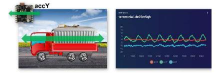
As expected, the movement was captured mainly in the *Y*-axis (green). In the blue, we see the *Z* axis, around  $-10 \text{ m/s}^2$  (the Nicla has the camera facing up).
