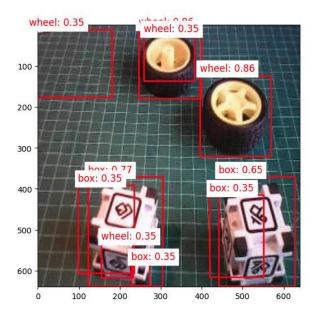
We start to see false positives and **multiple detections**, where the model detects the same object multiple times with different confidence levels and slightly different bounding boxes.
