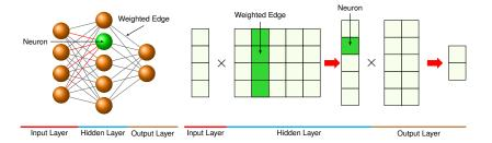
Figure 4.2: MLP layers and its associated matrix representation. Source: Reagen et al. (2017)
