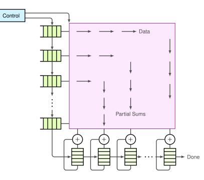
Figure 11.4: Data flow movement in a systolic array.
