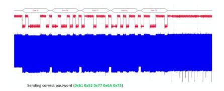
be incorrect, the device halts authentication. This change is reflected in the sudden jump in the blue power line, indicating that the device has stopped processing and entered an error state.
