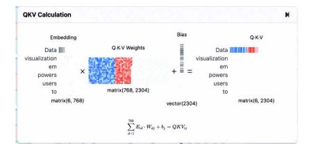
Figure 4.8: Dynamic weight calculation. Source: Transformer Explainer.
