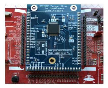
Figure 15.19: STM32F415 target board used in SCAAML experiments. Source: Bursztein et al. (2019).
