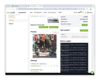
The latency of this model is approximately 86 ms, with an average power consumption of 420 mW.
