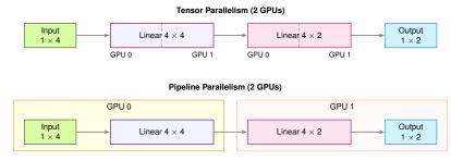
Figure 7.13: An example depiction of tensor parallelism versus pipeline parallelism. Note how the first case shards each Linear layer across GPUs, while the second assigns the first Linear to the first GPU and the second to the second GPU.
