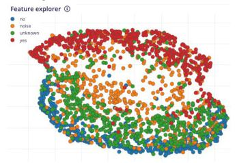
The result seems OK, with a visually clear separation between *yes* features (in red) and *no* features (in blue). The *unknown* features seem nearer to the *no space* than the *yes*. This suggests that the keyword *no* has more propensity to false positives.
