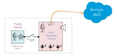
**Stage 1**: A small microprocessor inside the Echo Dot or Google Home continuously listens, waiting for the keyword to be spotted, using a TinyML model at the edge (KWS application).
