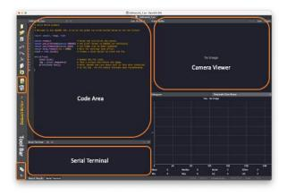
Any messages sent through a serial connection (using print() or error messages) will be displayed on the **Serial Terminal** during run time. The image captured by a camera will be displayed in the **Camera Viewer** Area (or Frame Buffer) and in the Histogram area, immediately below the Camera Viewer.
