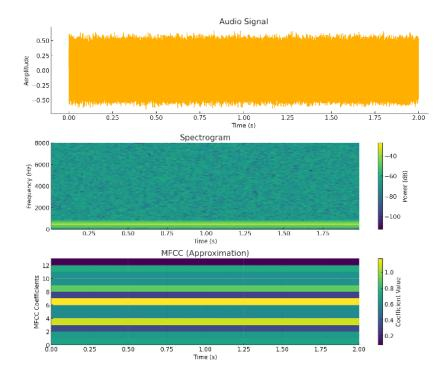
Figure 6.11: KWS data processing of an audio signal (top panel) represented in a spectrogram (middle panel) showing the energy distribution across time and frequency, along with the corresponding MFCCs (bottom panel) that capture perceptually relevant features.
