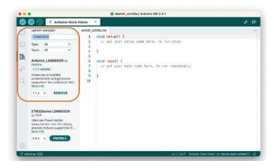
Next, go to Examples > Arduino\_LSM6DSOX > SimpleAccelerometer and run the accelerometer test. You can check if it works by opening the IDE Serial Monitor or Plotter. The values are in g (earth gravity), with a default range of +/- 4g:
