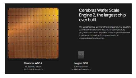
The Cerebras WSE is unlike traditional chips in that it is a single waferscale processor, spanning the entire silicon wafer rather than being cut into
