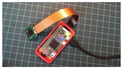
Here is another example of a v2 Camera Module, which has a **Sony IMX219** 8-megapixel sensor:
