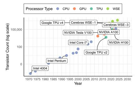
Figure 11.12: Processor transistor count over time.
