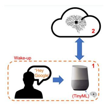
In other words, recognizing voice commands is based on a multi-stage model or Cascade Detection.
