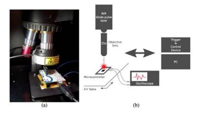
Figure 15.7: Laser fault injection attack on a microcontroller. Source: Breier et al. (2018).
