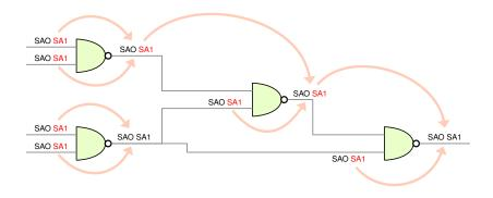
Figure 18.10: Stuck-at Fault Model in Digital Circuits. Source: Accendo Reliability
