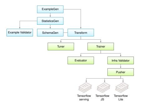
Figure 6.10: Example breakdown of the entire data to model processing pipeline for TensorFlow Extended.
