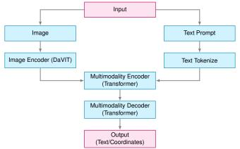
• **Image Encoder**: The image encoder is based on the DaViT (Dual Attention Vision Transformers) architecture. It converts input images into a series of visual token embeddings. These embeddings serve as the foundational representations of the visual content, capturing both spatial and contextual information about the image.
