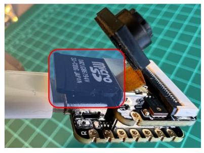
For a start, Insert the SD Card on the XIAO as shown in the photo below (the SD Card should be formatted to FAT32).
