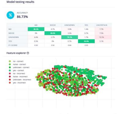
Inspecting the F1 score, we can see that for YES, we got 0.95, an excellent result once we used this keyword to "trigger" our postprocessing stage (turn on
