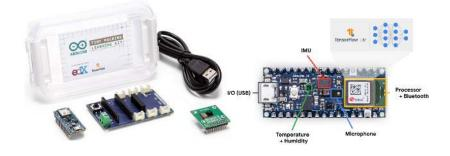
Figure 2.9: Examples of Tiny ML device kits. Source: Widening Access to Applied Machine Learning with Tiny ML.
