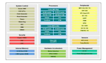
Note: Based on Seeed Studio documentation, besides the Himax internal memory of 2.5MB (2.4MB SRAM + 64KB ROM), the Grove Vision AI (V2) is also equipped with a 16MB/133 MHz external flash.
