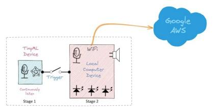
**Stage 1**: A smaller microprocessor inside the Echo Dot or Google Home **continuously** listens to the sound, waiting for the keyword to be spotted. For such detection, a TinyML model at the edge is used (KWS application).
