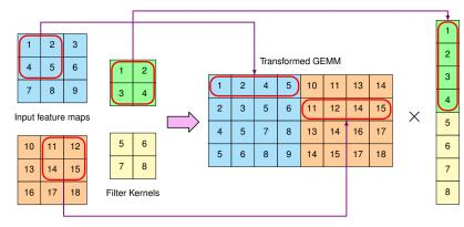
Figure 4.11: Depiction of how im2col can map a convolution into a dense matrix multiplication for better efficiency.
