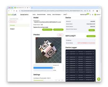
To run the Image Classification Model, the Grove Vision AI V2 had a peak current of 80mA at 5.24V, resulting in a **power consumption** of 420mW.
