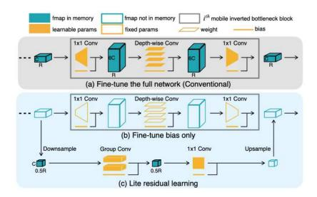
drastically reduced memory footprint. The frozen convolutional layers act as a fixed feature extractor, and only the trainable bias components are involved in adaptation. By avoiding storage of full activation maps and limiting the number of updated parameters, TinyTL enables on-device training under severe resource constraints.
