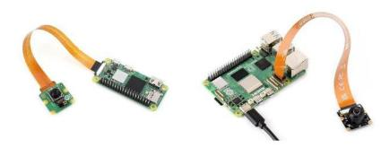
Figure 20.15: Raspberry Pi Zero 2-W and Raspberry Pi 5 with Camera
