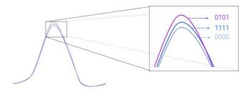
Figure 15.18: Power traces from an AES S-box operation. Source: Bursztein et al. (2019).
