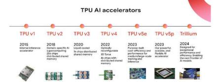
Figure 8.22: Tensor Processing Units (TPUs), a single, specific purpose chip desigend for accelerated AI.
