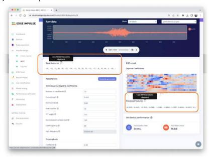
We will take the Raw features (our 1-second, 16 KHz sampled audio data) and use the MFCC processing block to calculate the Processed features. For every 16,000 raw features (16,000  $\times$  1 second), we will get 637 processed features (13  $\times$  49).
