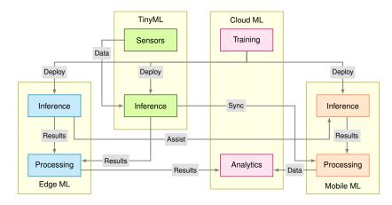
Figure 2.10: Example interaction patterns between ML paradigms, showing data flows, model deployment, and processing relationships across Cloud, Edge, Mobile, and Tiny ML systems.
