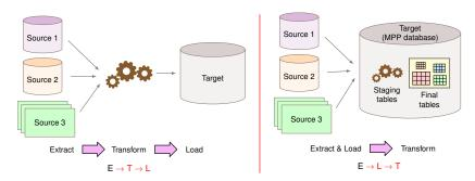
Figure 6.9: Key differences between Extract, Transform, Load (ETL) versus Extract, Load, Transform (ELT).
