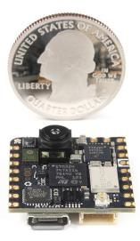
Figure 20.2: Nicla Vision. Source: Arduino
