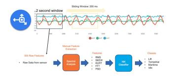
We can see 10 seconds of accelerometer data captured with a sample rate (SR) of 50 Hz. A 2-second window will capture 300 data points (3 axis  $\times$  2 seconds  $\times$  50 samples). We will slide this window each 200ms, creating a larger dataset where each instance has 300 raw features.
