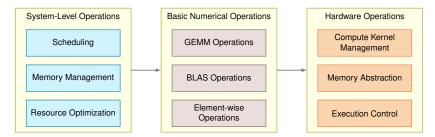
Figure 7.14: Hierarchical structure of operations in machine learning frameworks.
