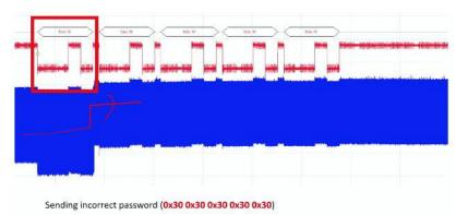
Figure 15.11: Power consumption profile of the device when an entirely incorrect password (0x30, 0x30, 0x30, 0x30, 0x30) is entered. The blue line shows a sharp jump after processing the first byte, indicating that the device has halted the authentication process. Source: Colin O'Flynn.
