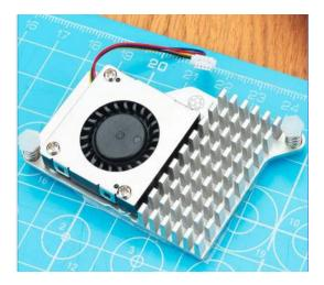
The Active Cooler has pre-applied thermal pads for heat transfer and is mounted directly to the Raspberry Pi 5 board using spring-loaded push pins. The Raspberry Pi firmware actively manages it: at 60°C, the blower's fan will be turned on; at 67.5°C, the fan speed will be increased; and finally, at 75°C, the fan increases to full speed. The blower's fan will spin down automatically when the temperature drops below these limits.
