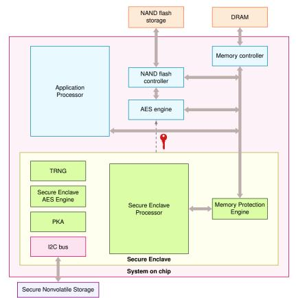
Figure 15.14: System-on-chip secure enclave. Source: Apple.
