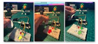
The power consumption reached a peak of 240 mA (Green LED), equivalent to 1.2 W. Driving the Yellow and Red LEDs consumes 14 mA, equivalent to 0.7 W. Sending information to the terminal via serial has no impact on power consumption.
