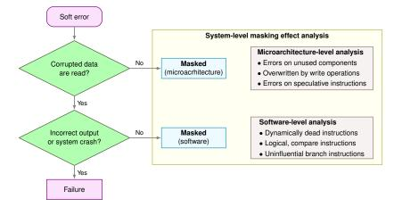
Figure 18.38: Example of error masking in microarchitectural components (Ko 2021)
