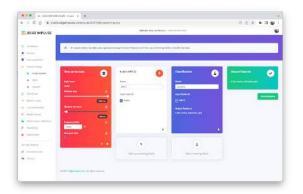
First, we will take the data points with a 1-second window, augmenting the data, sliding that window each 500 ms. Note that the option zero-pad data is set. It is essential to fill with zeros samples smaller than 1 second (in some cases, I reduced the 1000 ms window on the split tool to avoid noises and spikes).
