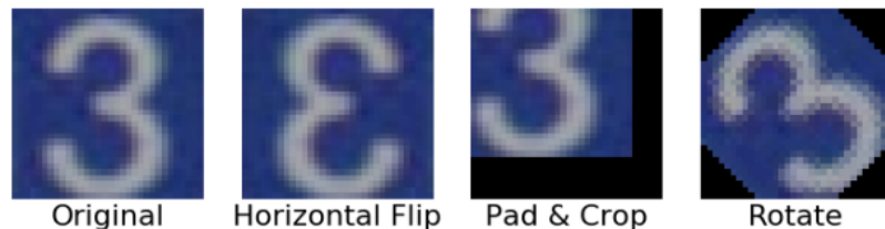
Figure 17.33.: An image of the number “3” in original form and with basic augmentations applied.
