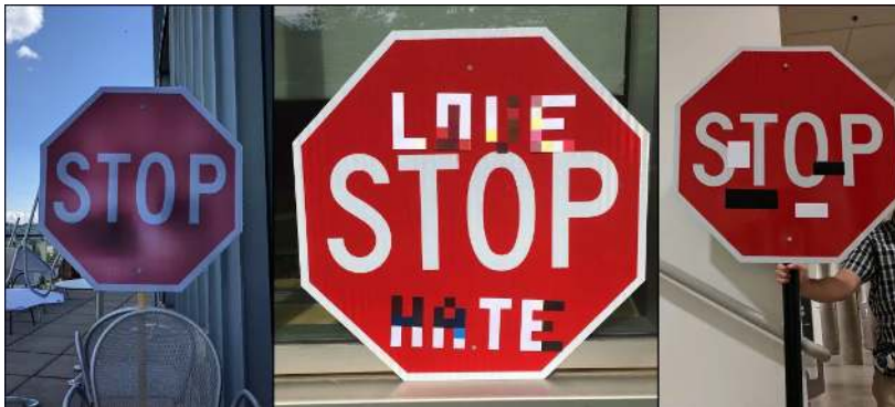
Figure 17.22.: Graffiti on a stop sign tricked a self-driving car into thinking it was a 45 mph speed limit sign. Source: Eykholt
