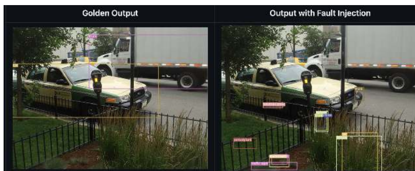
Figure 17.42.: Hardware bitflips in ML workloads can cause phantom objects and misclassifications, which can erroneously be used downstream by larger systems, such as in autonomous driving. Shown above is a correct and faulty version of the same image using the PyTorchFI injection framework.
